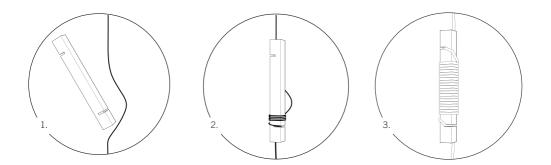
PLEASE NOTE! Always check if the cord is securely clamped inside bottom and top slit in the wooden pen (figure 3).
