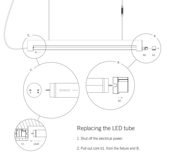
3. Take out the LED tube by carefully pulling at powered end while stopping the fitting from coming out of the hole (side C).
